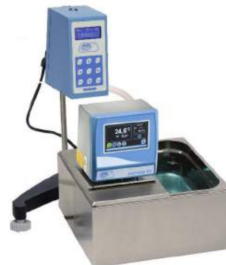
Use of a thermostat DIGITERM to control the temperature in viscosity measurement by means of the recirculation of the liquid.
